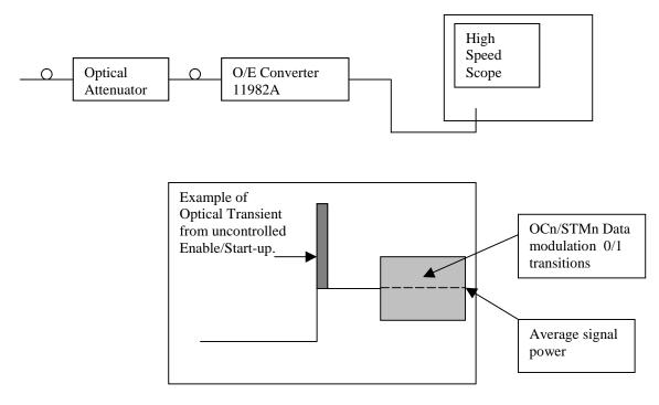
If excessive laser enable transients are observed then there is a need to ensure that Test Sets are protected by appropriate additional attenuation and the customer will of course want to investigate the reasons for any unexpected excessive transient from their equipment.
